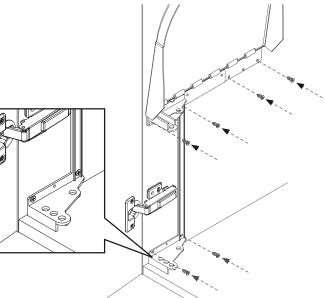
Fix the cover **G** on the mounting bar **C**.
